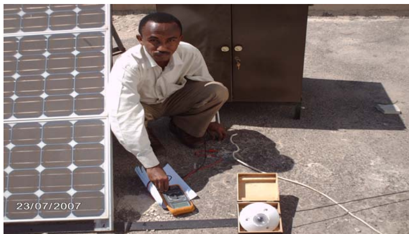
Figure (B.5) Measuring devices pyranometer and Avometer which were used in experiments.
