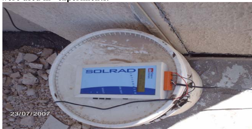
Figure (B.6) The integrator which was used to measure solar intensity during the experiment
