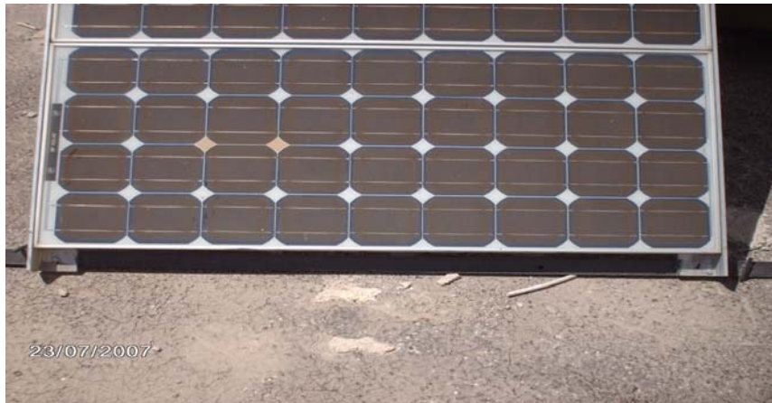
Figure (B.4) Photovoltaic panel of monocrystalline (one module).
